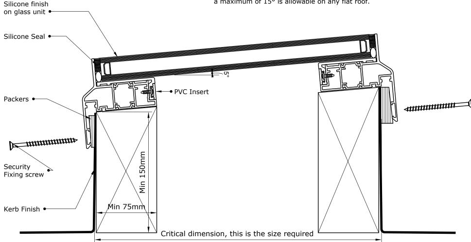
N.B. Roof, kerb, fixings, packers & kerb finishes are not provided
